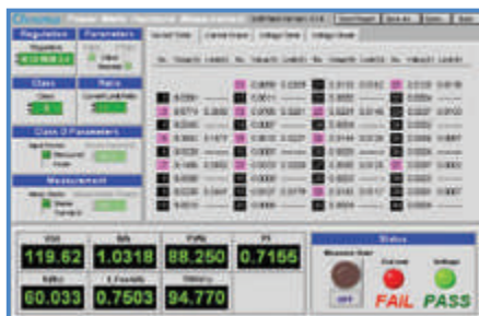
IEC 61000-3-2 Current Harmonics Test (Pre-compliance)
